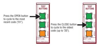
The operator will only keep track of up to 20 codes, then will start saving over the oldest codes as new codes occur.
